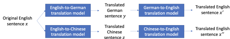
Figure 5: The data augmentation workflow of CERT using back-translation. Image taken from [FWZ + 20].
